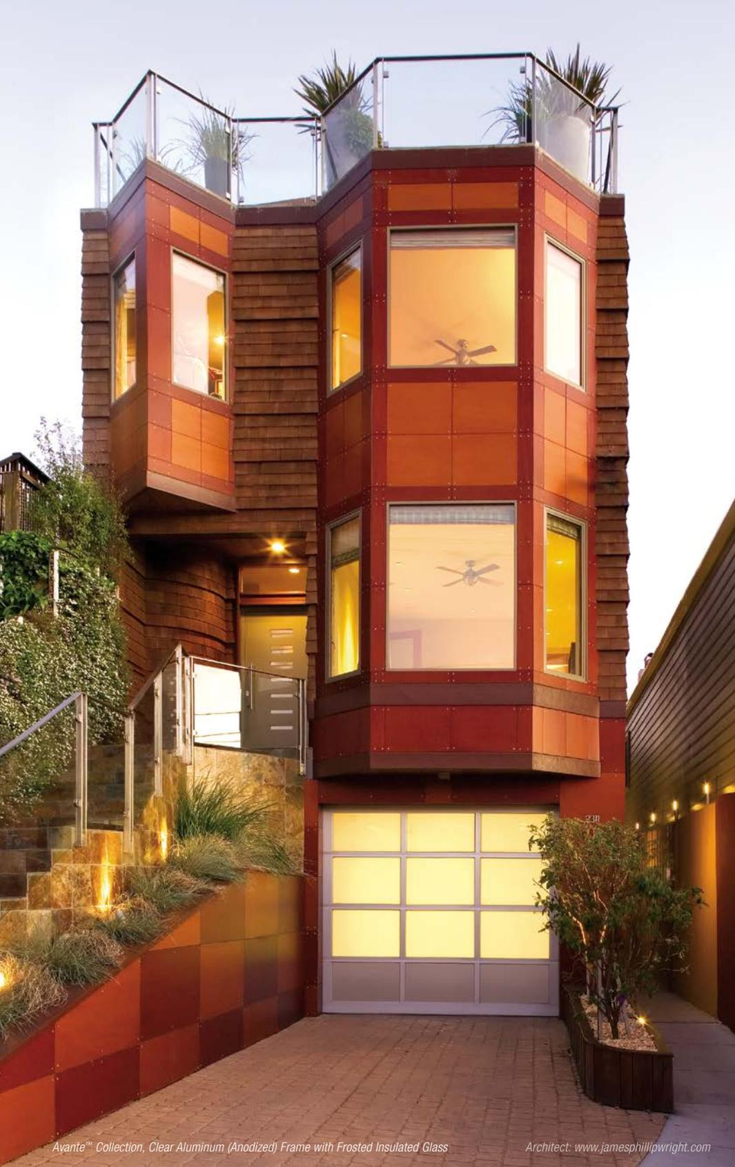
Avante™ Collection, Clear Aluminum (Anodized) Frame with Frosted Insulated Glass
